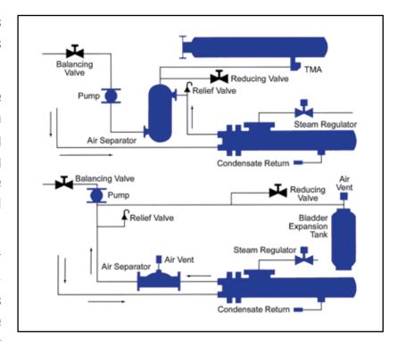
system; however, the capacity of the boiler must be sufficient to handle the load imposed by the heat exchanger. In addition, some method of controlling the flow to the exchanger must be provided and installed according to the manufacturer's directions.
